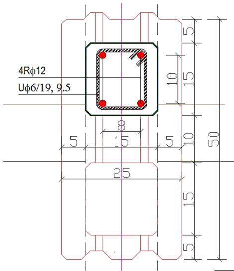
Section of concrete inside a column in Simprolit block SBDN-25
